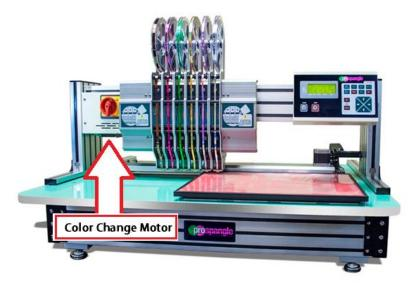
2) To the left of the Motor look for the metal Dial © and turn it slowly so the press units begin to move towards the right, keep turning until the error beeping stops and the error disappears from the screen.
